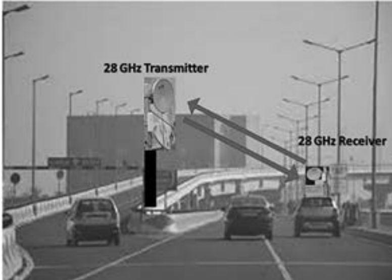
Figure 7.12 (a) RFID tag on vehicle used for device discovery use cases. (b) Prototype installation of 28 GHz communication system with one unit mounted on Roadside UNIT (RSU) and 2nd Unit on Vehicle.
